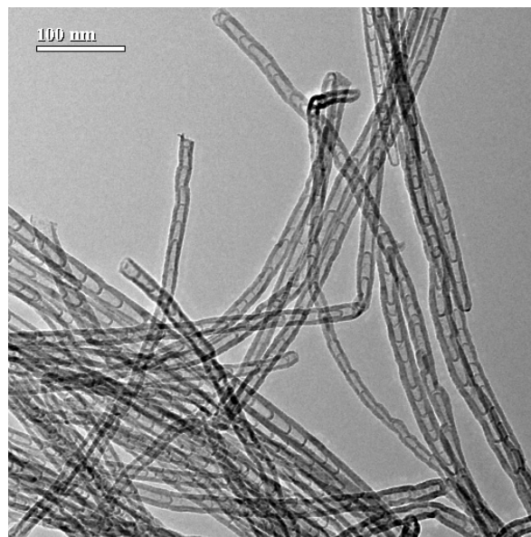
Figure 1: TEM image of MWCNTs with an average diameter of 20 nm (with permission of Dr Bill Li).
