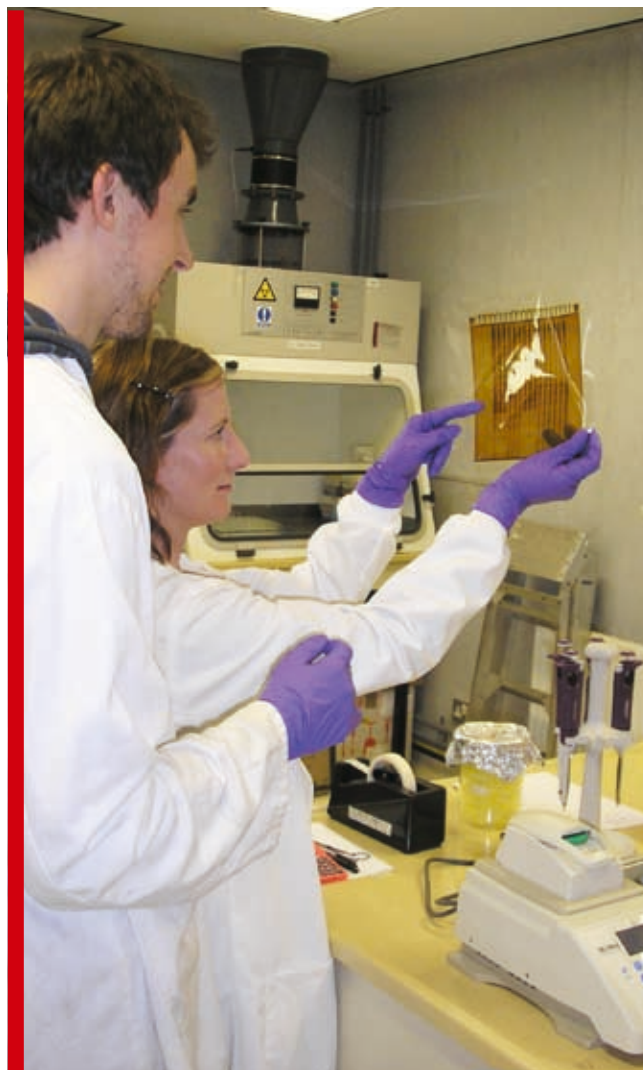
Dr Liz Shaw (University of Reading) and PhD student Laurence Cullen examine the effect of nanoscale zerovalent iron (nZVI) on soil microbial communities using a denaturing gradient gel electrophoresis image.
