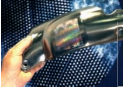
The Institute for New Materials (INM) in Saarbrücken has developed nanoparticle processes for applying counterfeit-proof, wear-resistant holograms to metal components.
