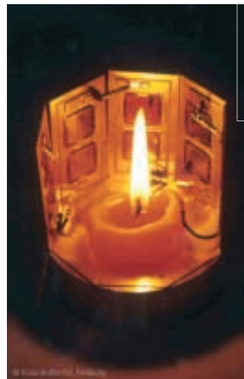
Candlelight is enough for thermo-photovoltaic cells to produce enough power to operate a radio.
