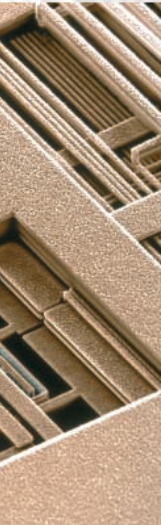
As complex as a miniature city – etched copper circuits of a chip (IBM), viewed with the aid of a scanning electron microscope. Modern chips have up to nine circuit levels.
