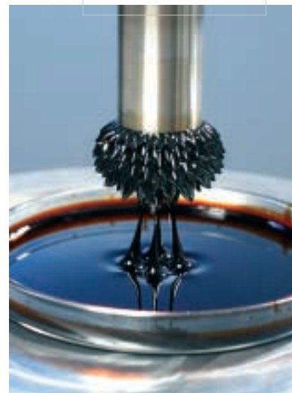
Magnetite nanoparticles in oil. The fluid can be controlled and shaped magnetically.
