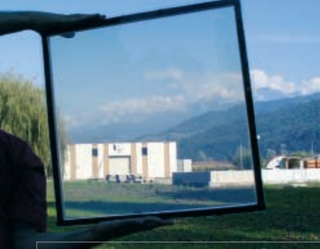
Double-glazing filled with an aerogel reduces heat losses.
