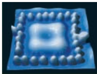
Manganese atoms on silver at the Christian-Albrechts University of Kiel. The electrons enclosed by the cage of manganese atoms form distribution patterns, which depend on the electrical voltage applied. Effects such as this will be important for the electronics of tomorrow.
