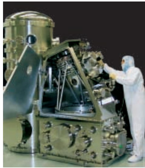
Prototype of an EUV wafer-stepper system for the production of future chip generations.
