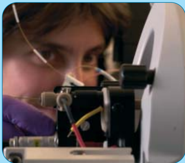
Microchromatographic column. © P. Stroppa, CEA
