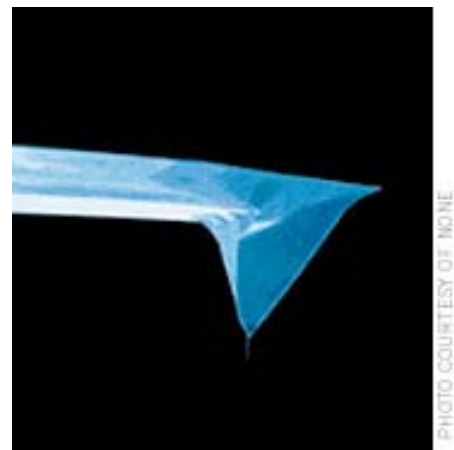
Figure 5: The tip of an AFM. Adapted from Mirkin et al. www.chem.nwu.edu/~mkngrp/dippen.html
